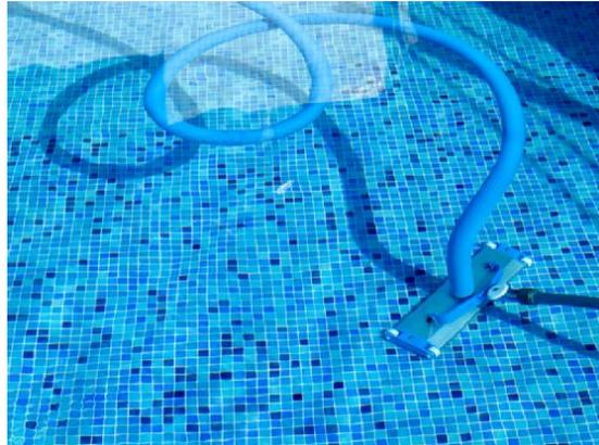
Sediment and some dirt may find their way to the floor of the pool and will need to be removed with a swimming pool vacuum cleaner. The swimming pool vacuum cleaner works in the same manner a household unit does except that instead of drawing air, it draws water.
